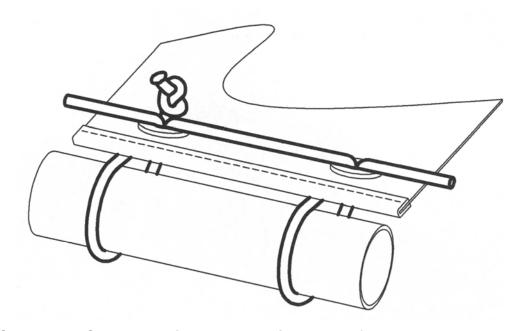
Completed Canopy Lacing and Knotting: When finished your lacing and knotting should look like this.
